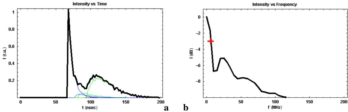
**Fig. 3:** Figure 3a shows the impulse response of the channel corresponding to the illumination pattern example in Figure 2a corresponding to an arbitrary arrangement of source/detector directivity angles. Thin lines in (a) give impulse responses between individual source/detector pairs before summing. Figure 3b shows the frequency response for the impulse response in 3a. The + in 3b indicates the 3dB point of the channel response. Intensity is in relative units.
