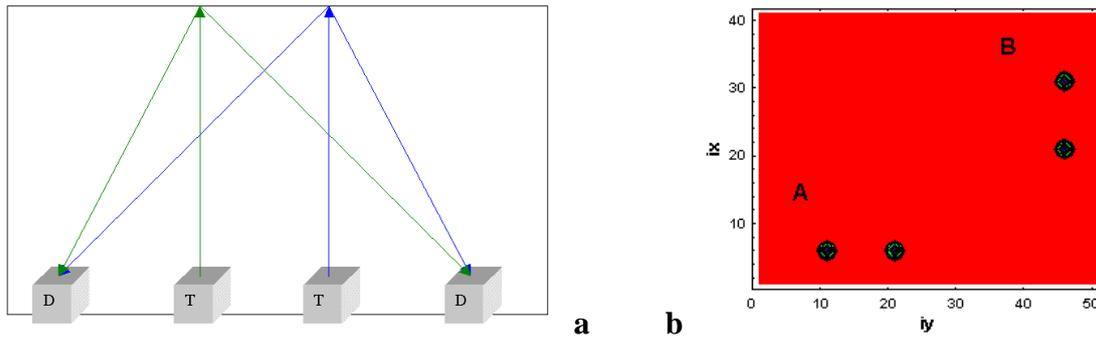
**Fig. 1:** (a) gives the cross-section diagram of a room for the IR channel model. The transmitters (T) and detectors (D) interact via reflections from the ceiling only. Figure (b) on the right indicates the positions of two specific sets (A,B) transmitter/detector pairs on the floor of a 4x5 meter room (axes in dm) with a 2m high ceiling. These give our simulation geometry.
