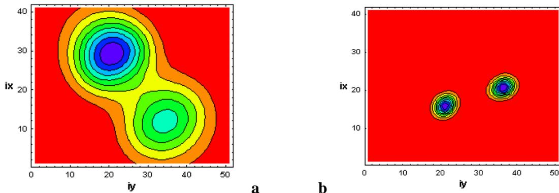
**Fig. 2.** (a) and (b) above indicate the detected IR light patterns by set B when set A is transmitting in the two cases corresponding to an arbitrary and optimized, respectively, beam/FOV angles and widths discussed in the next section. The parameter  $n$ , defining the width of the beams, are chosen to be between 5–20 for case (a) and between 100–200 for case (b).
