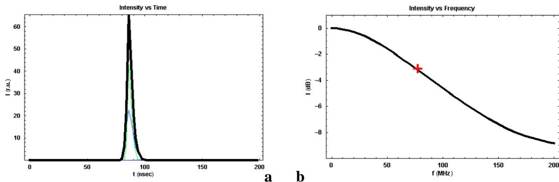
**Fig. 4:** Figure 4a shows the impulse response of the channel after optimization of source/detector directivity angles and widths. Figure 4b shows the frequency response and indicates the 3dB point of the channel bandwidth.
