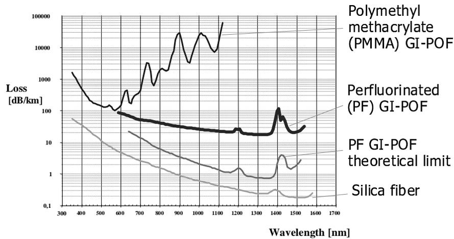
Fig. 1: Attenuation of GI-POF
