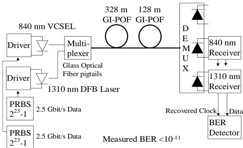
Fig. 2: Block diagram of the 2 times 2.5 Gbit/s over 456 m PF GI-POF CWDM transmission experiment.
