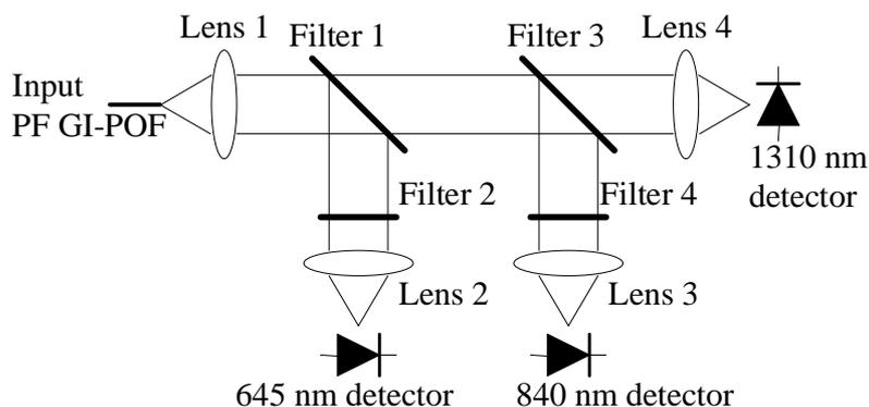
Fig. 3: Principle of operation of the 645, 840, 1310 nm demultiplexer.
