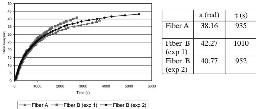
Figure 4: (a) Measured phase shift as a function of the time; (b) Exponential fit on the measured data with a the magnitude of the shrinkage and the time constant  $\tau$
