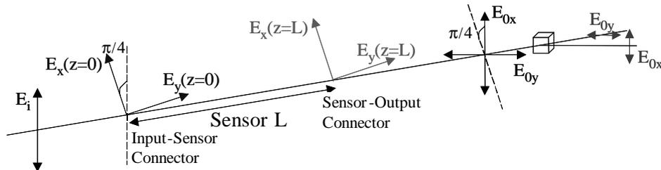
Figure 2: Polarimetric sensor configuration
