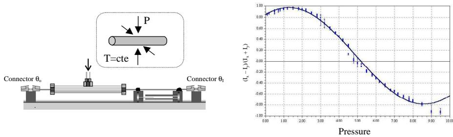
Figure 3: (a) Experimental set-up for measuring the pressure sensitivity; (b) Sensor response as a function of the pressure (HB800, L= 35 cm)
