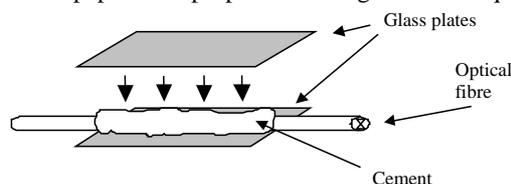
Figure 1: Three-layered configuration with the dental cement between 2 glass plates
