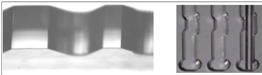
**Figure 3 :** Photographs of uniform cylindrical micro lenses and optical fiber alignment grooves.
