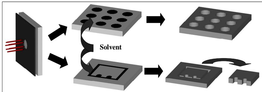
**Figure 2 :** The basic proces steps for the fabrication of micro hole arrays and more complex 2 1/2D structures.
