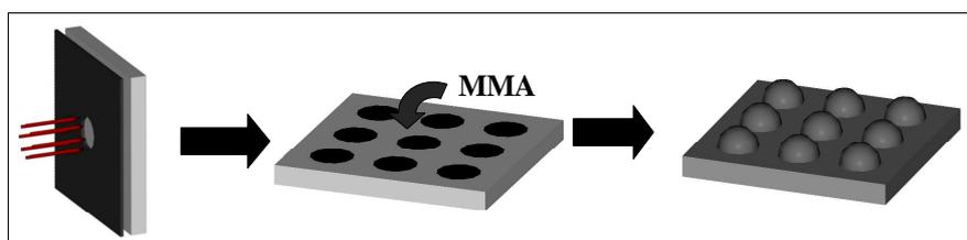
**Figure 1 : Basic process steps for the fabrication of stable and uniform spherical micro-lenses.**
