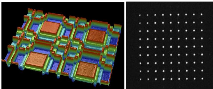
Figure 4 3D profiles of DOE with a 1x81 fan-out (on the left) and its output intensity distribution.
