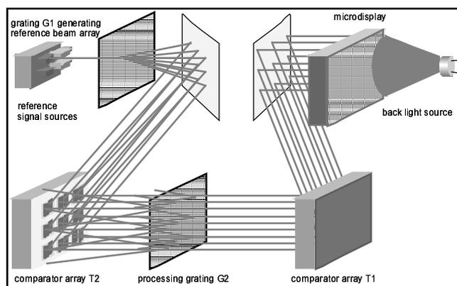
Figure 1 The functionality scheme of a photonic local image processor.
