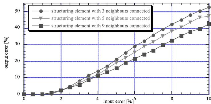
Figure 3 The influence of input image non-uniformities on the output signal in the presence of structuring elements with 3, 5 and 9 connected neighbours
