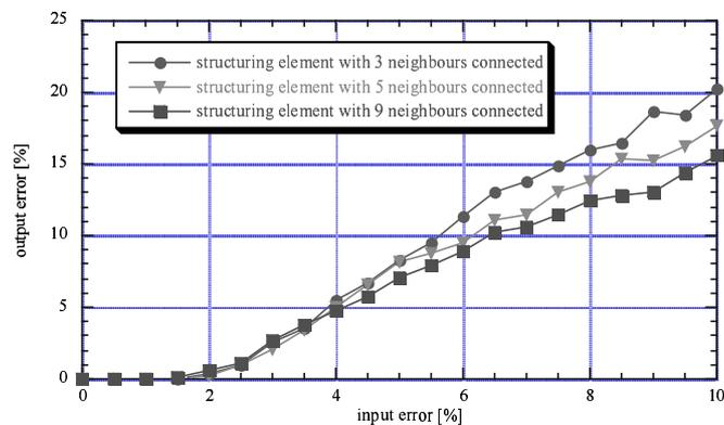
Figure 2 The influence of structuring element non-uniformities with 3, 5 and 9 connected neighbours on the output signal..
