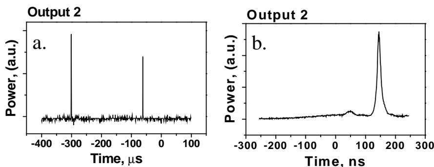
**Figure 2.** Typical oscilloscope traces recorded at pump power of 80 mW (basic laser configuration, a - large x-scale, b – small x-scale).
