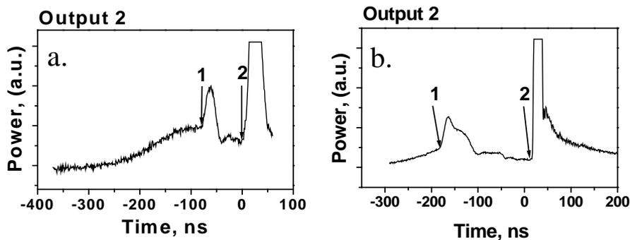
**Figure 3.** Fine structure of laser pulses at pump power of 80 mW (a - basic laser configuration, b – configuration with long linear cavity).
