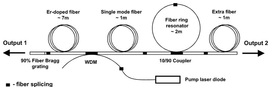
**Figure 1.** Experimental setup (lengths of fibers are indicated for the basic configuration).
