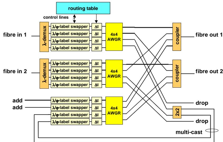
**Fig. 4 2x2 Label-controlled router with 4x4 AWGRs**
