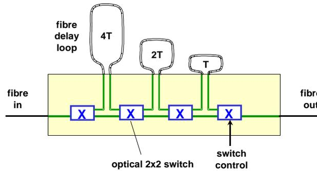
**Fig. 3 Switchable delay line**
