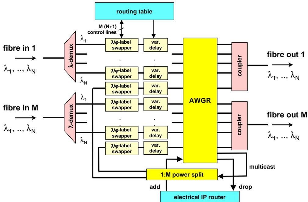
**Fig. 2 Optical label-controlled router**
