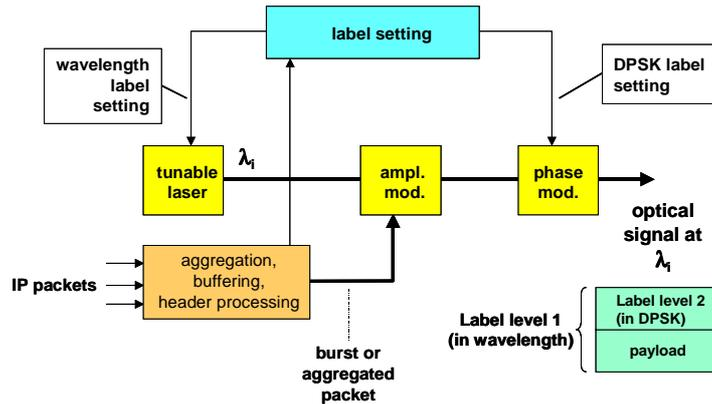
**Fig. 1 Two-level optical labeling in edge router**
