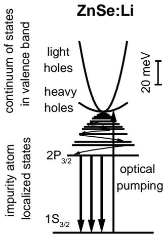
**Fig. 2.** Scheme of optical (vertical arrows) and non-radiative transitions for ZnSe:Li. THz lasing (arrows down) is expected from the  $2P_{3/2} \rightarrow 1S_{3/2}$  optical transitions.  $2P_{3/2}$  is acceptor long-living state.
