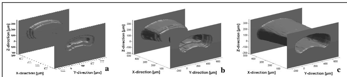
Figure 2: Simulation of the etching profile of a curved irradiated line after three arbitrary timeframes
