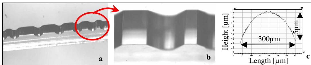
Figure 3: A close-up of a cylindrical micro-lens array with different chords and ultra-small heights.
