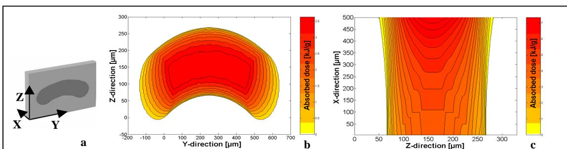
Figure 1: The absorbed dose profiles at the top surface (b) and a cross section at  $Y = 250\mu\text{m}$  (c) after a curved line irradiation.
