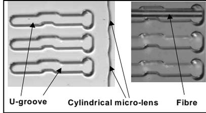
Figure 4: Top view of the monolithic integration of cylindrical micro-lenses with U-grooves and the positioning of optical fibres by mechanical alignment features.
