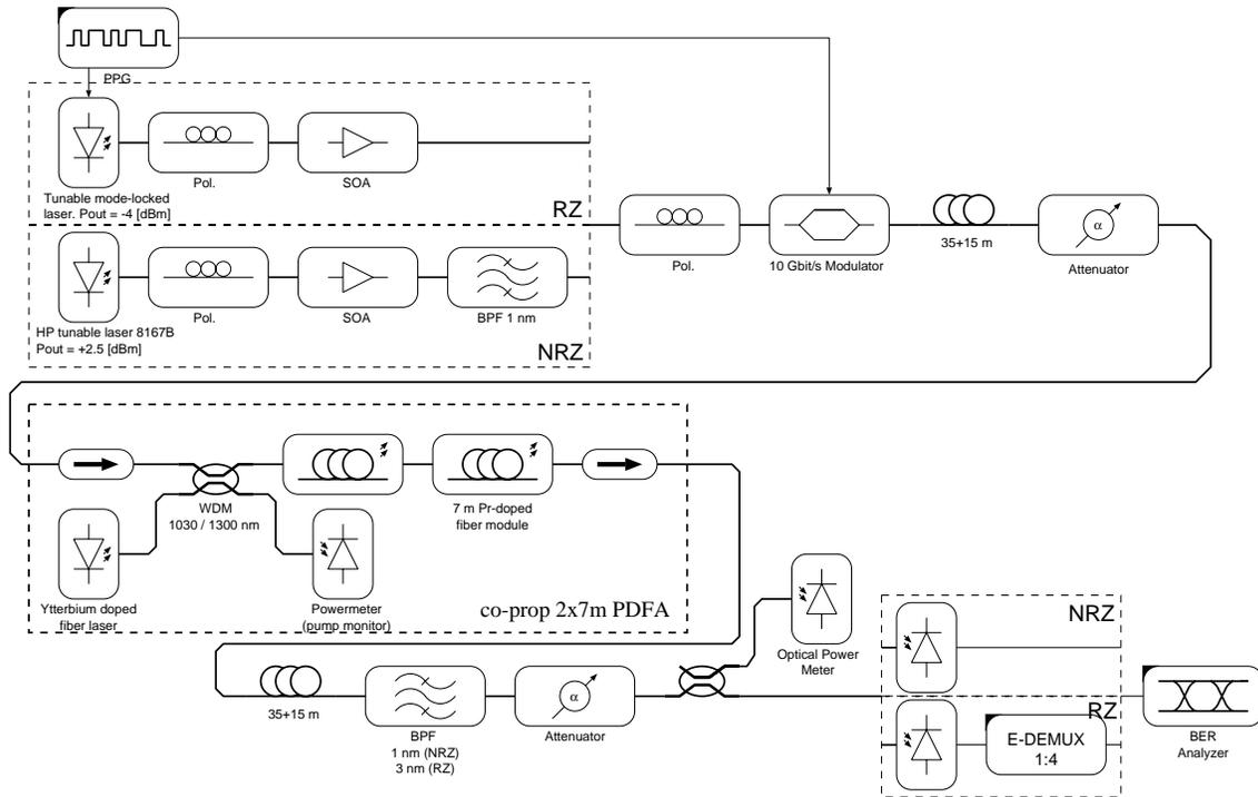
Figure 1: Experimental setup for performance assessment of PDFA in copropagating configuration.
