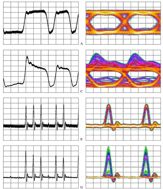
Figure 3: Pattern- en Eye-diagrams for PDFA (A,B,E and F) and SOA (C,D,G and H).
