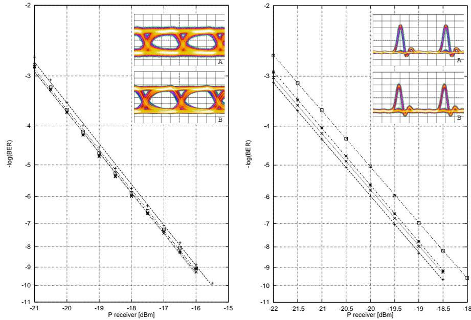
Figure 2: BER measurements for 10 Gbit/s NRZ (left) and RZ (right) at 1300 nm. (+) B2B, (X)  $P = -5$  [dBm], (\*)  $P = -10$  [dBm] and (□)  $P = -15$  [dBm].
