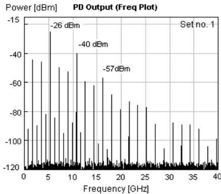
Figure 4: RF Spectrum at the Output of the Photodiode
