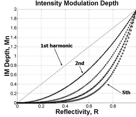
Figure 3: Intensity Modulation Depth of Harmonic Components
