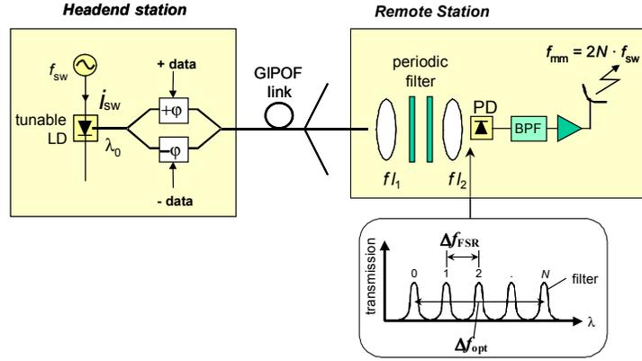
Figure 1: Generating Modulated Microwave Signals via Polymer Optical Fiber Links
