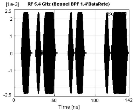
Figure 5: Time plot of Electrical Signal Filtered at 5.4 GHz
