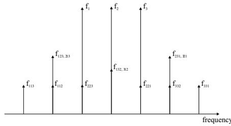
Figure 1: Example of the FWM effect for three co-propagating waves
