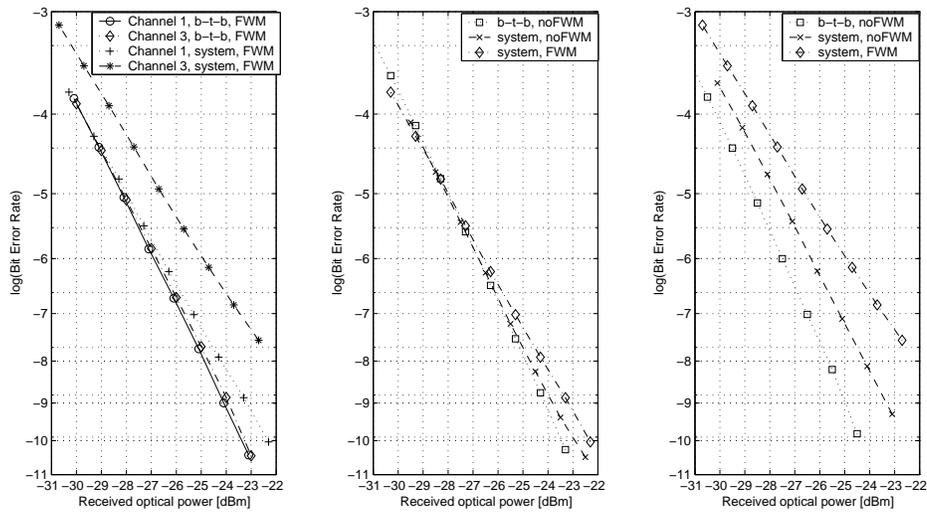
Figure 4: BER measurements graphs. The left graph: channel 1 and channel 3, equal channel spacing. The middle graph: channel 1, equal and unequal channel spacing. The right graph channel 3, equal and unequal channel spacing
