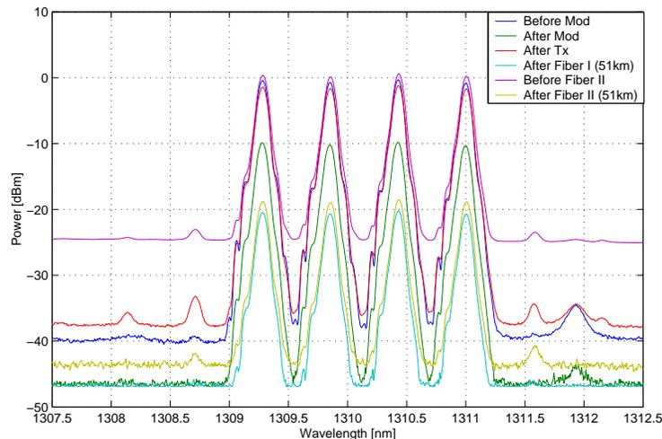
Figure 3: Evolution of the signal power in the experimental set-up. (Lowest wavelength channel 1, highest wavelength channel 4)
