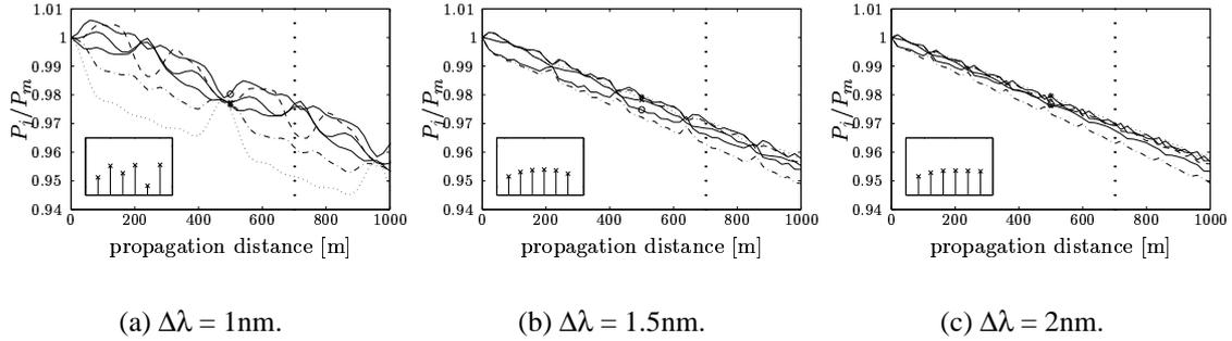
Figure 3: Normalized power evolution of 6 WDM channels at  $1.55\mu\text{m}$ ,  $L = 1\text{km}$ ,  $P_m = 8\text{mW}$  in a SMF for different channel spacings. For (a), the channels are mismatched at the input of the fiber. The dotted lines indicate where the spectral power distributions shown in the insets are measured.
