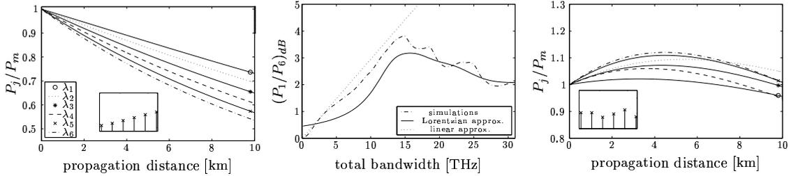
(a) Normalized power evolution of 6 WDM channels at  $1.55\mu\text{m}$ ,  $D = 16.7\text{ps/nm/km}$ ,  $L = 10\text{km}$ ,  $P_t = 48\text{mW}$  (17dBm) and  $\Delta\lambda = 8\text{nm}$ . The insets show the output spectral power distribution at 10km.  $(P_1/P_6)_{dB} = 1.36\text{dB}$ ,  $\Delta P = 47 \times 10^{-4}$ .
