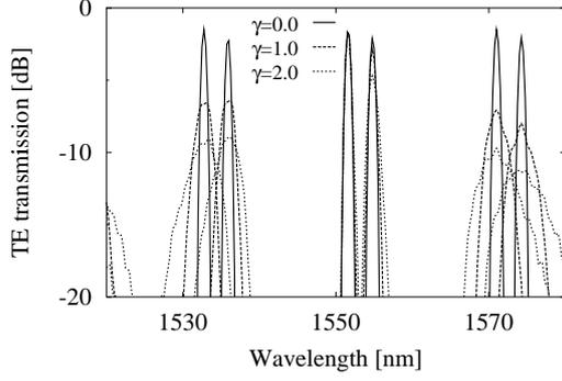
Figure 2: *Simulated transmission spectra of the chirped phased-array for three chirp factors  $\gamma$ .*
