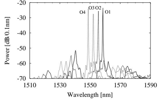
Figure 3: *Spectra from the multiplexed output of the separately biased channels of the chirped MWL.*
