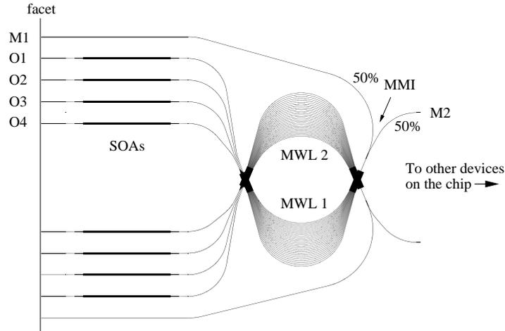
Figure 1: Two chirped phased-array based MWLs with 4 channels. The SOAs have been integrated monolithically with passive waveguides and can be identified as the thick lines on the left side of device.
