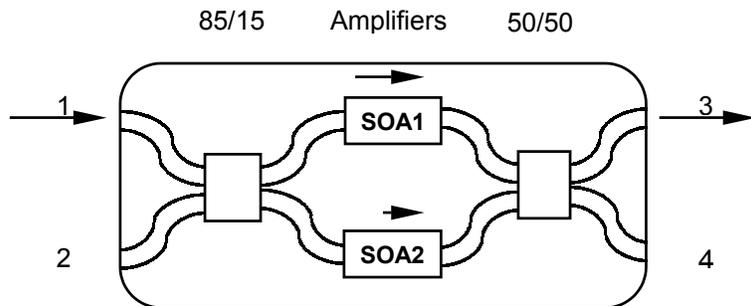
Fig. 2. Schematic layout of the pattern effect compensator.
