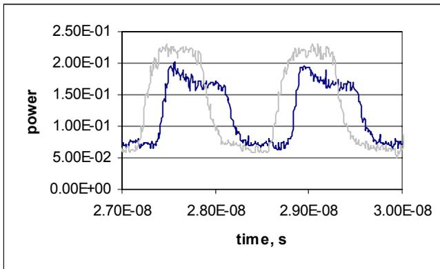
Fig. 7. Compensated (light line) and uncompensated (dark line) waveforms for an input power of  $-0.54$  dBm (0.88 mW).
