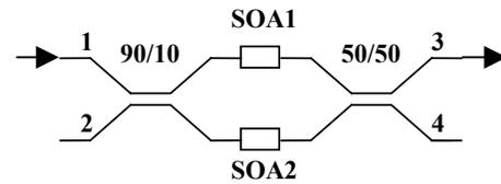
Fig. 6. The MZI-structure used in the experiments.
