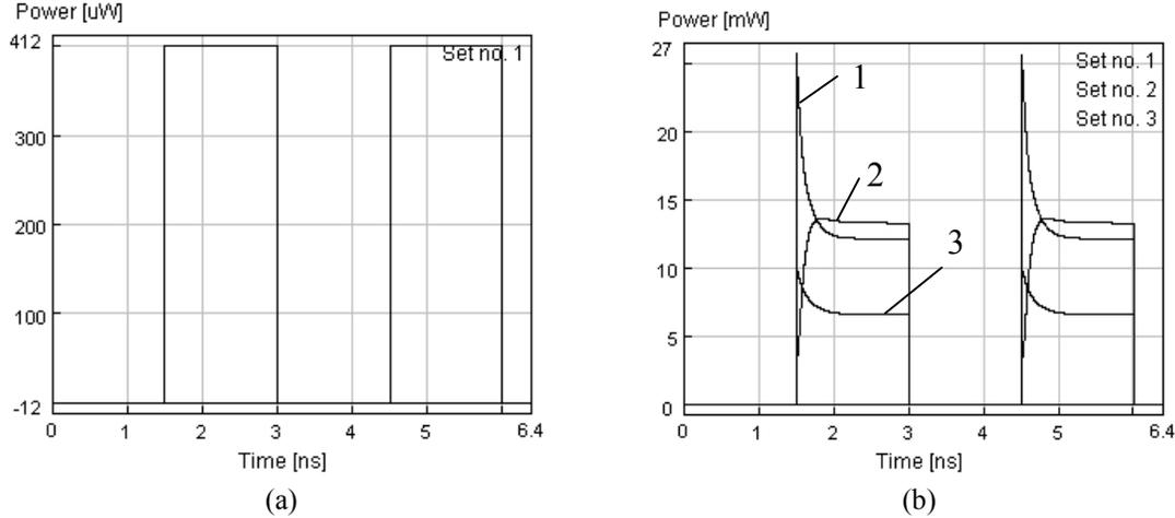
Fig. 4. Input (a) and output (b) pulses of the interferometric structure and SOAs. Curves: 1-output of SOA used in the branches of MZ-interferometer, 2-output of the compensator, 3-output of a SOA with the equal to the device small-signal gain.
