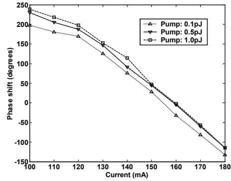
**Figure 3:** Simulation of the phase change of a 20 fJ probe pulse as a function of the injection current for various pump pulse energies.
