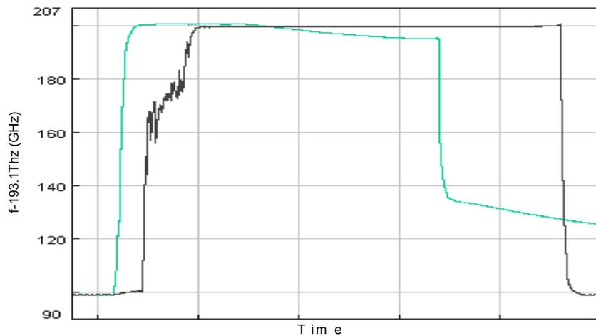
Fig. 7: Frequency switch for the laser with (—) and without (—) feedback
