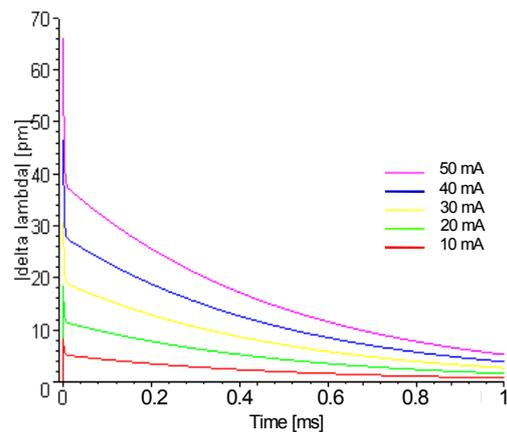
Fig. 2: Drift for increasing current step
