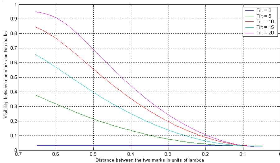
Figure 3: Visibility between one mark and two marks for the coupling to the first-order mode of the waveguide. The different ascending curves are for different tilts of the waveguide varying from  $0^\circ$  (lower curve) to  $20^\circ$  (higher curve). Calculation parameters:  $W = 2 \lambda$ ,  $n_{co} = 3$ , scan height =  $1 \mu\text{m}$ ,  $\lambda = 0,9 \mu\text{m}$ .
