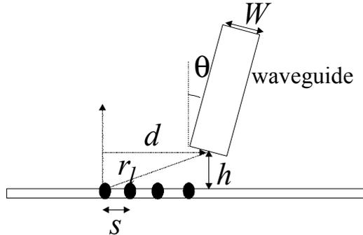
*Figure 1: Outline of the model for detection of an array of point sources (thick dots) using a multimode waveguide of width  $W$  which is scanned at a height  $h$  from the point sources. The position of the waveguide with respect to the sources is given by  $d$  where  $d=0$  coincides with the first source on the left. The waveguide is tilted by an angle  $\theta$  with respect to the source plane.*
