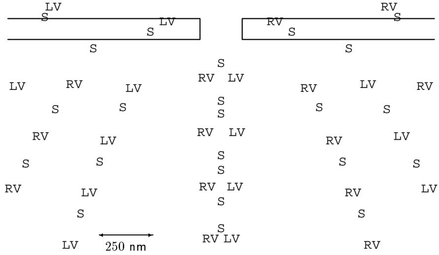
Figure 2: Location of phase singularities in the field of power flow near a 200 nm wide slit in a 100 nm thick silver plate. The incident light (coming from below) has a wavelength  $\lambda = 500$  nm. The left- and right-handed optical vortices are denoted by lv and rv, respectively. s denotes a saddle point.
