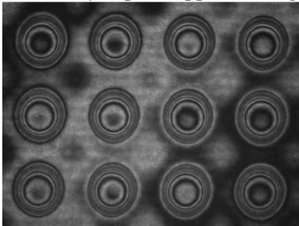
Figure 5: Spherical wave illumination of the prototyped PMMA baseplate showing the lens uniformity. The pitch is 175  $\mu\text{m}$ , diameter 122  $\mu\text{m}$  and the average height is 10.3  $\mu\text{m}$ .
