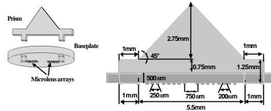
Figure 2: The dimensions of the OIM
