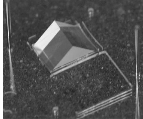
Figure 4: Prototype OIM with mechanically aligned glass prism. The second glass prism is to be aligned in front of it using visual/active alignment.
