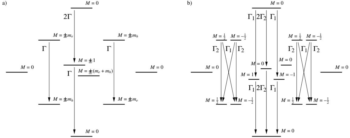
Figure 2: Two different schemes for cylindrical dots. a) In the case  $|m_e - m_h| = 1$ , the exciton multiplet consists of a bright and a dark doublet. b) For the case  $m_e = m_h = \frac{1}{2}$ , the exciton level is split into a doublet and two singlets. One singlet is a dark state. This results in six optical emission frequencies.
