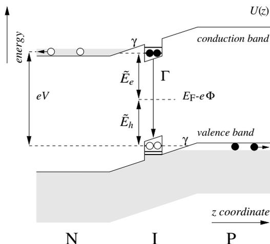
Figure 1: Energy-band structure of the PIN junction, for a cross section through the quantum dot along the  $z$  axis. The quantum dot is a small cylindrical structure located in the I layer between N and P semiconductors. With the gate potential  $\Phi$ , the electron and hole energies can be shifted. A bias voltage  $V$  over the junction allows electrons (black) and holes (white) to tunnel across the barriers with rate  $\gamma$  and  $\Gamma$  is the photon emission rate, as indicated.
