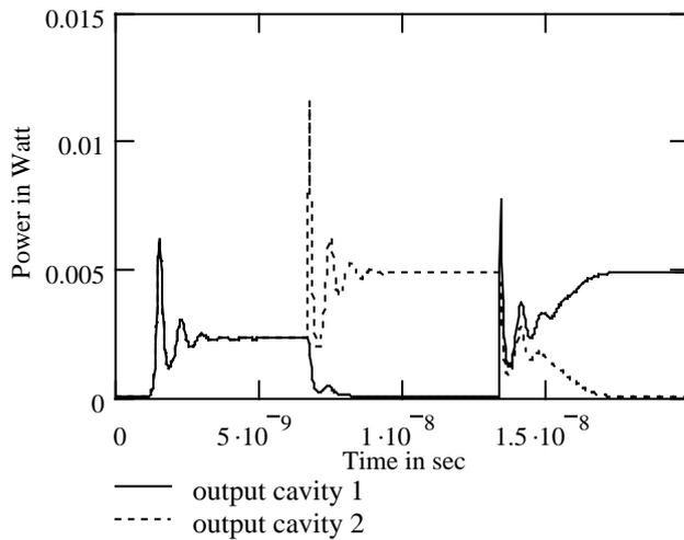
Figure 2. Output power of the memory system as a function of time with a 50ps set pulse and reset pulse.
