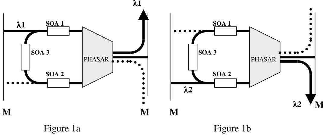
Figure 1. Schematic overview of the optical memory cell based on two coupled cavities in its two stable states, producing output at  $\lambda_1$  (a) or  $\lambda_2$  (b).
