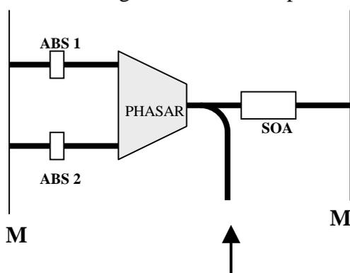
Figure 3. A diagram showing the memory cell based on a tunable laser with saturable absorbers.
