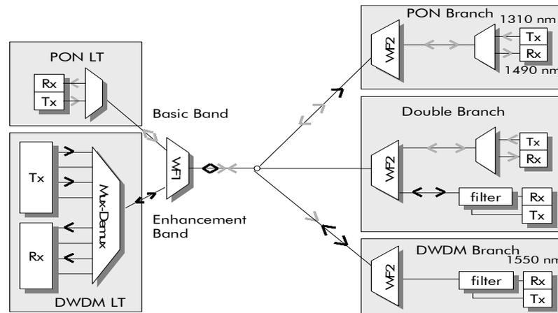
**Figure 1: DWDM overlay PON based upon a power splitter.**
