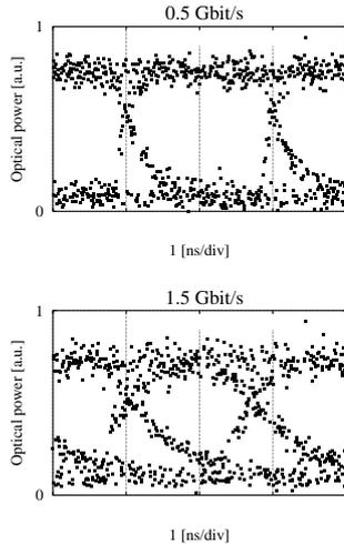
Figure 3: Eye patterns of the integrated device.
