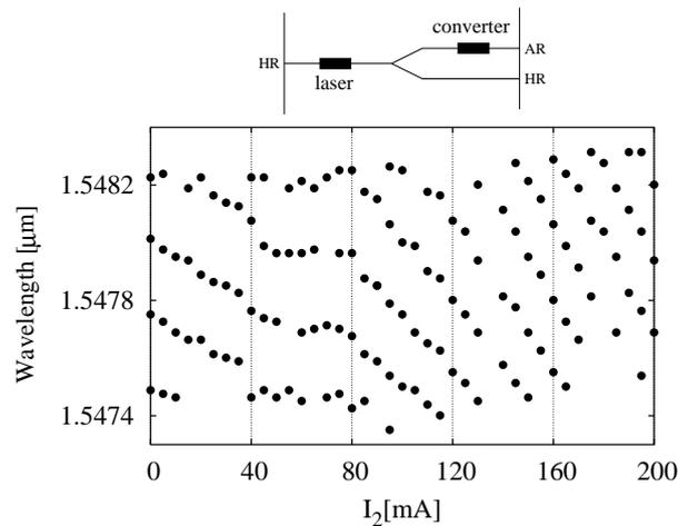
Figure 4: Position of wavelength peaks of the laser as function of the current in converter  $SOA_2$ .
