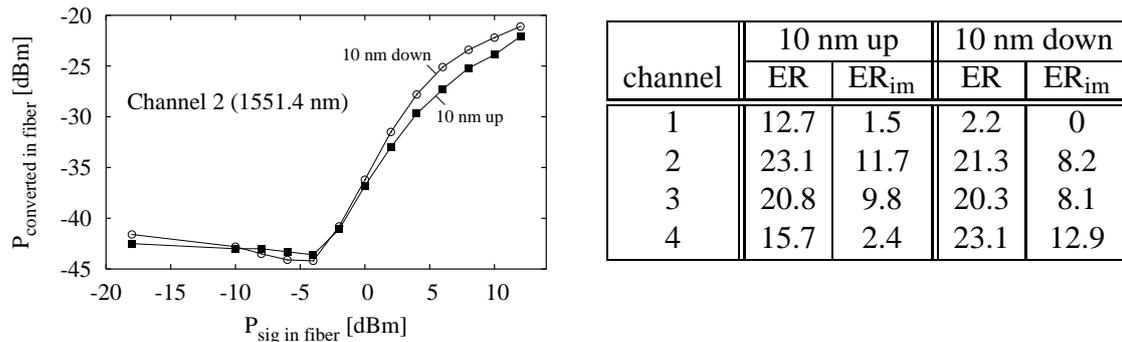
Figure 2: Wavelength conversion (non-inverting) (left) to channel 2 of the MWL from 10 nm shorter and longer signal wavelengths. SOA injection currents were:  $I_1 = 100$  mA,  $I_2 = 175$  mA,  $I_{pre} = 75$  mA. (right) Output ERs (ER) and best case ER improvements (ER<sub>im</sub>) of both 10 nm up conversion and 10 nm down conversion.
