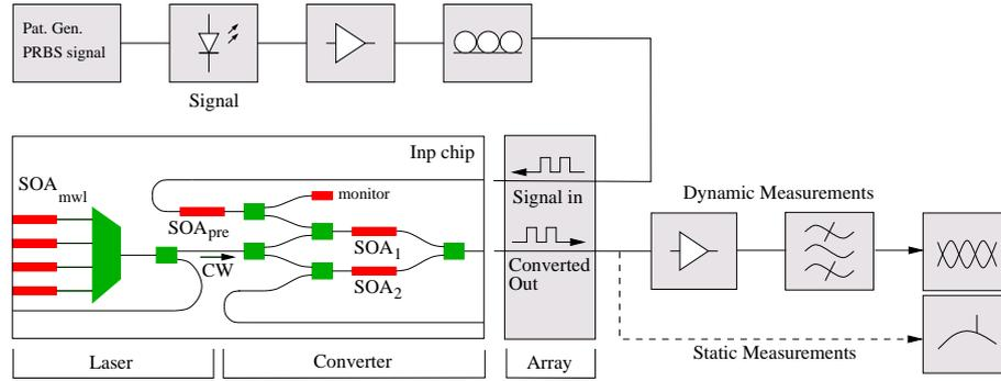
Figure 1: *Measurement set-up and circuit scheme of the MZI wavelength converter with a 4-channel PHASAR multi wavelength laser.*
