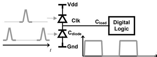
Figure 1: Schematic view of the receiver-less direct clock injection.
