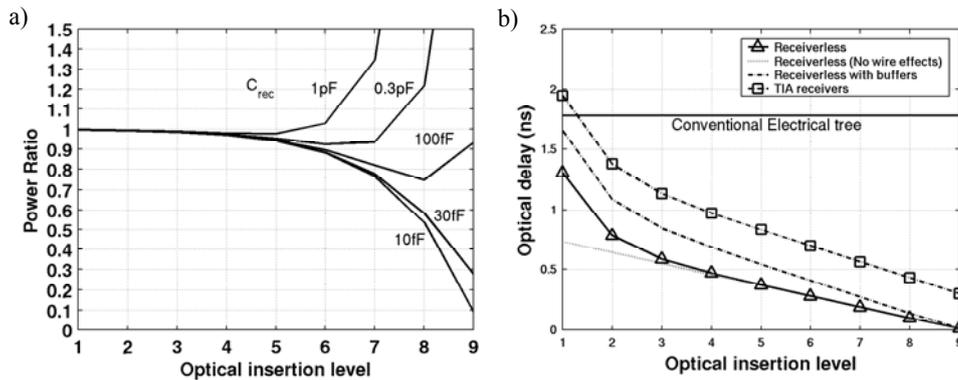
**Figure 3: Modeling of the optical clock distribution a) The power consumed in the distribution tree and b) The total delay of the distribution**
