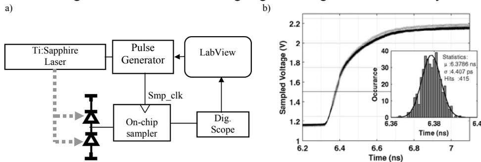
**Figure 2: a) Schematic view of the set-up b) A jitter plot showing the result of the sampled rising edge of the MQW totem pole. The subplot shows the histogram of the signal at the 1.5V crossing point.**
