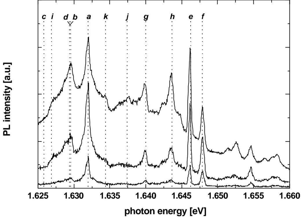
Fig. 1.: Three  $mPL$  spectra, taken at excitation densities of 16, 64 and  $640 \text{ W/cm}^2$ , respectively. The transitions labeled ‘a’, ‘e’ and ‘f’ emerge at low excitation and are identified as ground state (11) and excited state (12, 21) single-exciton recombinations. The bi-exciton transition is labeled ‘b’. The other peaks increase nonlinearly with excitation density. The dashed vertical lines are fits to the spectrum, see Table I.
