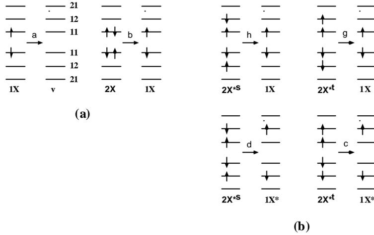
Fig. 2. (a) Ground state exciton  $1X @ v(\text{vacuum})$  and bi-exciton  $2X @ 1X$  recombinations, showing the ground (11) and excited (12) and (21) QD-states. Spin states are represented by vertical arrows. (b) Various relevant excited  $2X$  transitions. Superscripts 's,t' indicate singlet and triplet configurations. Labels 'a' - 'h' are assigned in Table I.
