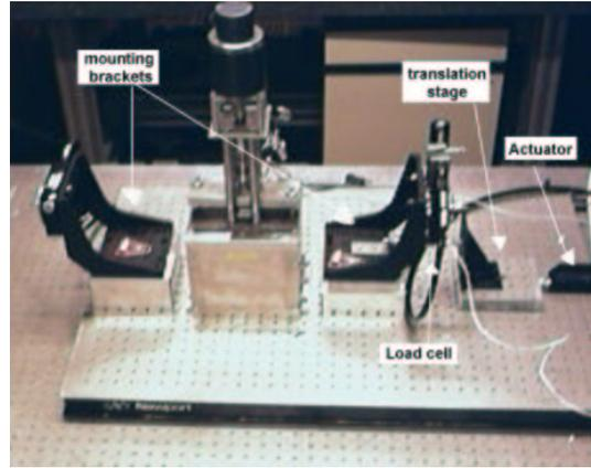
Figure 1: Multi-axial calibration set-up for multi-parameter FBG sensors
