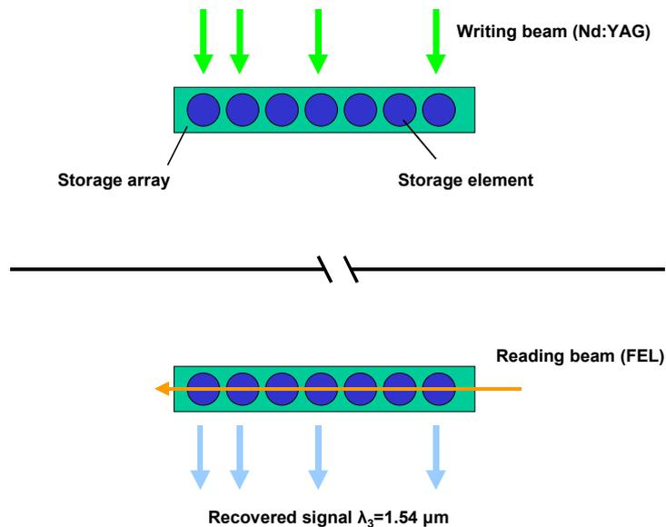
Fig. 2. Schematic illustration of "all-silicon" optically memory element based on the described optical memory effect.
