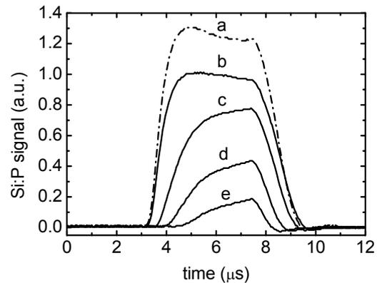
Fig. 4. Pulse shape of the Si:P stimulated emission for different pump intensities under direct excitation of the  $2p_0$  state.
