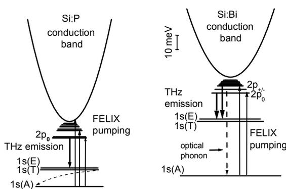
Fig. 1. Energy level schemes of Si:P and Si:Bi
