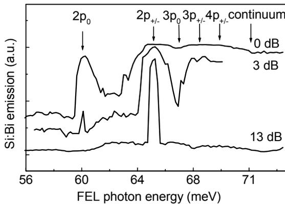
Fig.3. Si:Bi. Stimulated emission as a function of the frequency at different FELIX pump powers.
