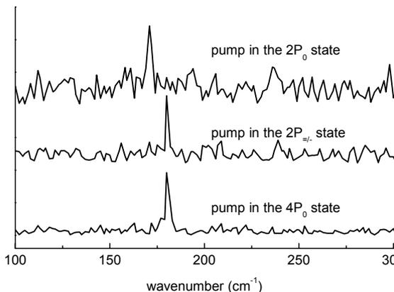
Fig. 5. Si:P: Spectra of the stimulated emission, optically exciting different donor states.
