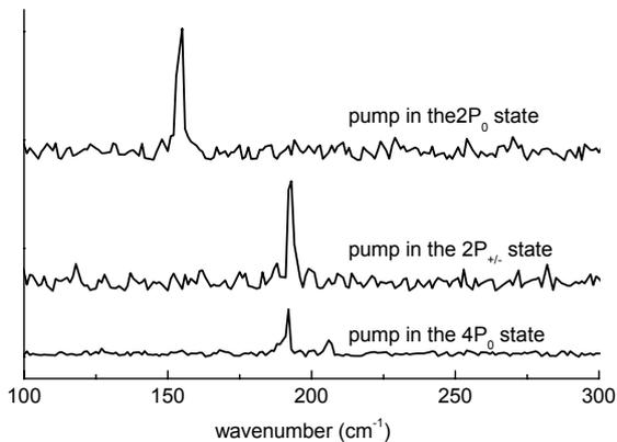
Fig. 6. Si:Bi: Spectra of the stimulated emission, optically exciting different donor states.
