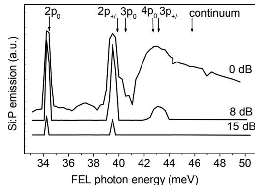
Fig. 2. Si:P Stimulated emission versus frequency at different FELIX pump powers.
