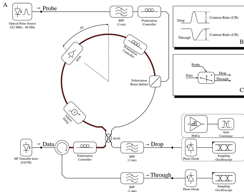
Figure 2: A) Experimental setup for performance assessment of a Terahertz Optical Asymmetrical Demultiplexer (TOAD) (BPF Band Pass Filter, SOA Semiconductor Optical Amplifier, PDFFA Praseodymium Doped Fibre Amplifier). B) TOAD output signals envelope. C) Functional block representation of TOAD.
