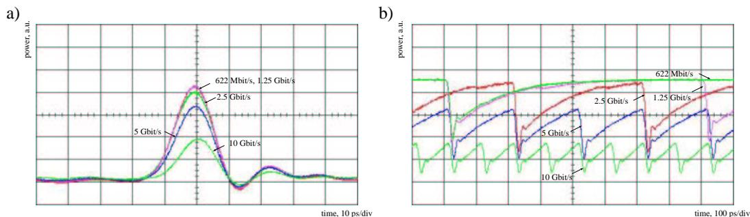
Figure 3: Switch characteristics of the drop (a) and through (b) channel for different optical granularities.
