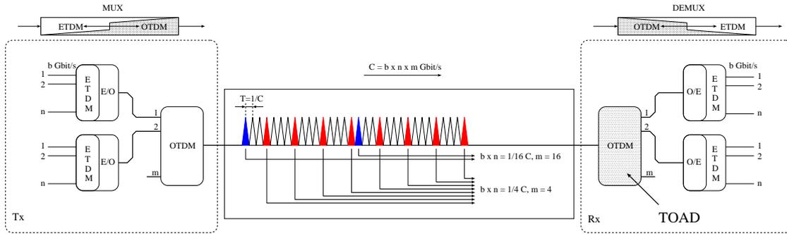
**Figure 1:** Schematic overview of point-to-point transmission system using Optical and Electrical Time Domain Multiplexing with transmission capacity  $C = b \times n \times m$  Gbit/s, with  $b$  ETDM granularity,  $n$  number of electrical tributaries of ETDM signal and  $m$  number of optical tributaries of OTDM signal (O/E optical-to-electrical conversion)
