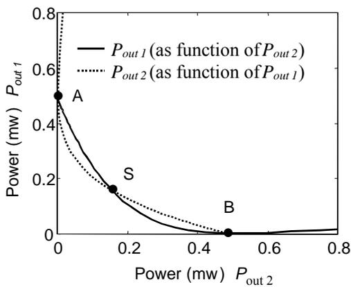
**Figure 2.** Intensity  $P_{out 1}$  of the light that outputs PSW<sub>1</sub> as a function of the intensity  $P_{out 2}$  of the light that outputs PSW<sub>2</sub> (solid curve). Intensity  $P_{out 2}$  of the light that outputs PSW<sub>2</sub> as a function of the intensity  $P_{out 1}$  of the light that outputs PSW<sub>1</sub> (dashed curve). It is clear that the two curves are complementary.
