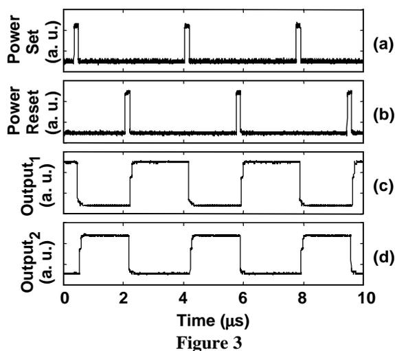
**Figure 3.** Dynamic output of the flip-flop showing switching between states every 1.85  $\mu$ s. The upper panels (Figure 3a and Figure 3b) are the traces of the external optical pulses at wavelength 1552.52 nm. The lower panels (Figure 3c and Figure 3d) are the dynamic output of flip-flop at output<sub>1</sub> ( $\lambda_1=1549.32$  nm) and output<sub>2</sub> ( $\lambda_2=1550.92$  nm).
