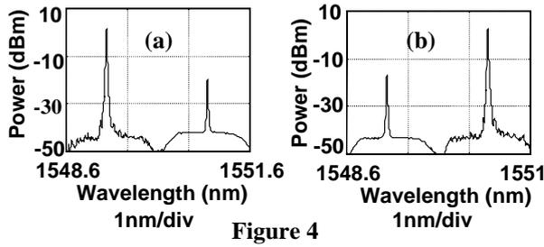
**Figure 4.** Spectral output at each state of the flip-flop. Figure 4a represents State 1 (wavelength  $\lambda_1$  1549.32 nm dominant), and Figure 4b represents State 2 (wavelength  $\lambda_2$  1550.92 nm dominant).
