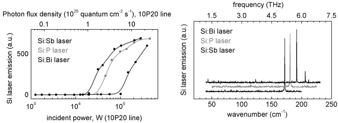
**Fig. 2.** Left graph: Dependences of the Si laser outputs on the pump power for the 10.6  $\mu\text{m}$  pump line. Right graph: Si laser emission spectra for the 10.6  $\mu\text{m}$  pump line (10P20).
