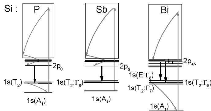
**Fig. 1.** Scheme of optical (vertical) and non-radiative transitions in Si lasers pumped by a CO<sub>2</sub> laser radiation. THz lasing (arrows down) occurs from the intracenter donor transitions.  $2p_0$  is donor long-living state in Si:P and Si:Sb. Resonant depletion of the  $2s$  and  $2p_{\pm}$  state by an optical phonon forms the population inversion in Si:Bi.
