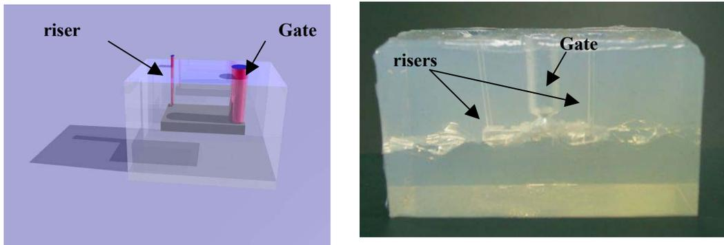
Figure 1 Rubber mold configuration: a. Drawing, b. Image with two risers and one gate in the middle
