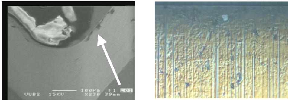
Figure 5 a. SEM image of small metal particles on the edge of the moldinsert, b. colored interference measurement of replica to show scratches on the surface
