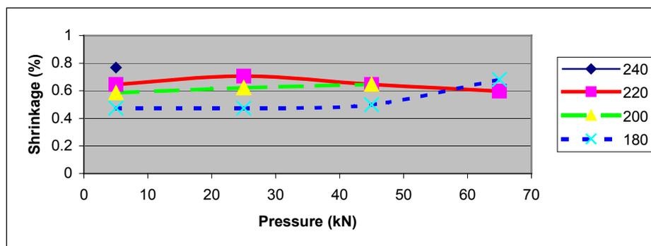
Figure 4 Shrinkage at different pressures and temperatures
