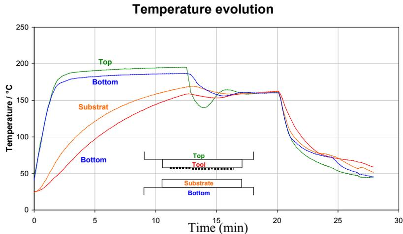
Figure 3 Heating cycle of hot embossing
