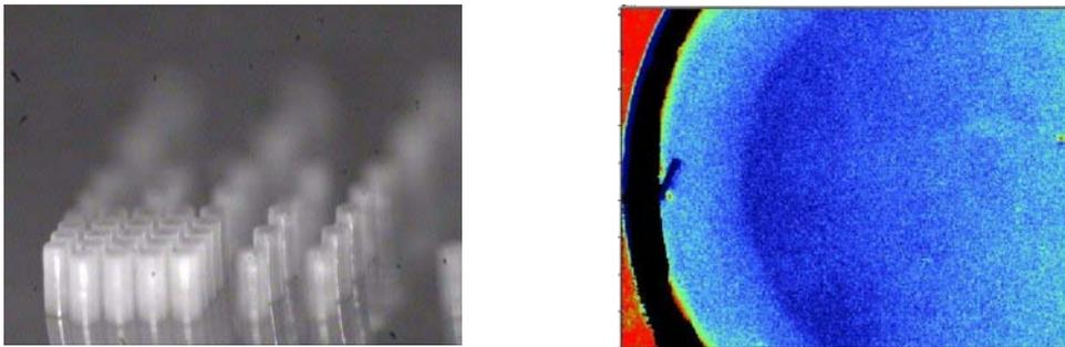
Figure 2 a. Rubber pins (500 $\mu\text{m}$  height, 200 $\mu\text{m}$  diameter), b. Height profile of an oxide-confined teststructure for vcsel fabrication
