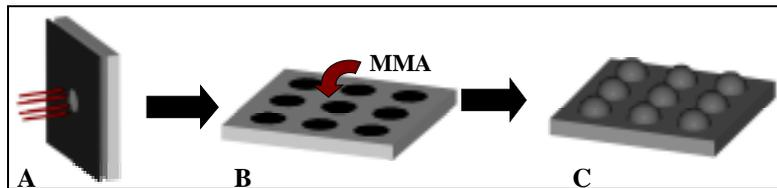
**Figure 2:** The basic processing steps for the fabrication of 2D arrays of stable and uniform spherical micro-lenses (C): Irradiating the PMMA-layer through an accurate pinhole (A) and applying a MMA-vapour on the surfaces of the irradiated sample (B).
