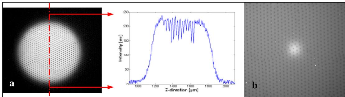
**Figure 5:** Images of an 800µm (a) and 50µm (b) 10 MeV proton beam, delivered by the LNS Tandem, with a SFOP that allows for real-time beam analysis.
