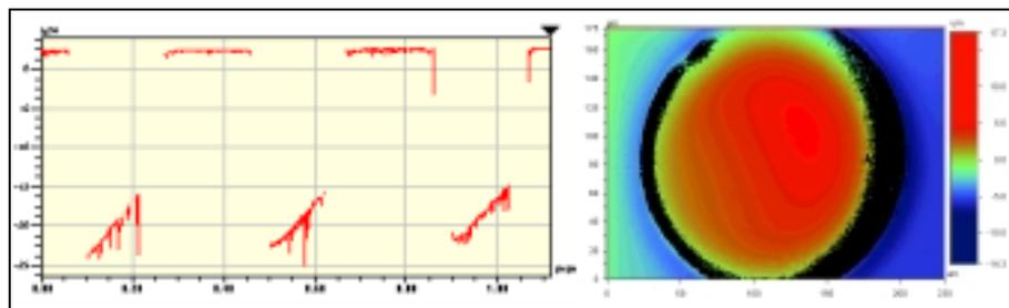
**Figure 3:** Tilted etching surfaces (a) and shifted lens tops (b) as a direct effect of inhomogeneous ion densities.
