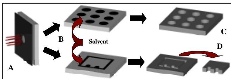
**Figure 1:** The basic processing steps for the fabrication of micro-hole arrays (C) and more complex 2 1/2 dimensional structures with high optical surface quality (D): Irradiating the PMMA-layer through an accurate pinhole (A) and etching the irradiated zones in a selective solvent (B).
