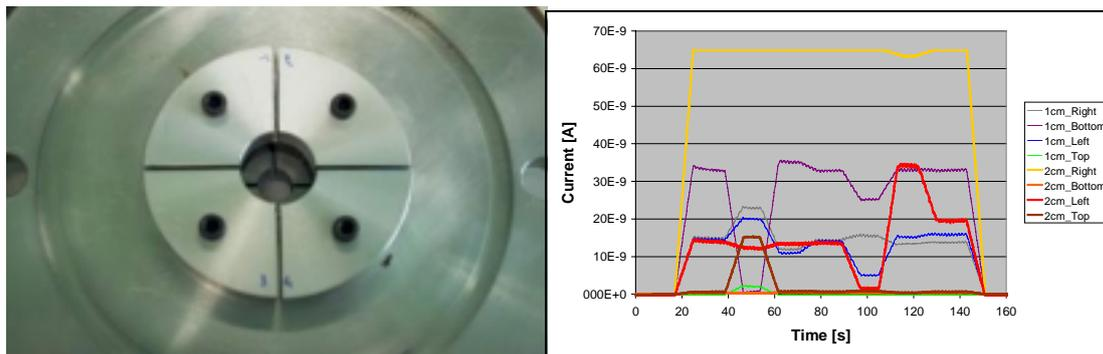
**Figure 4:** Construction of an 8 segment beam monitor (a) and resp. current measurements with individual picoammeters (b).
