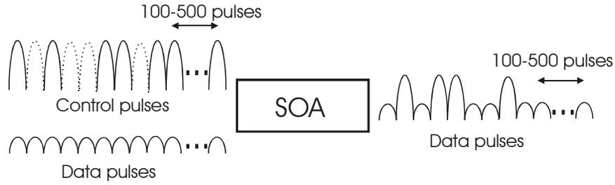
**Figure 1:** Control and data pulses configuration for simulation of data pulse evolution, where a serial of the control pulses train: 1010011011 is introduced after repetitive 100-500 pulses.
