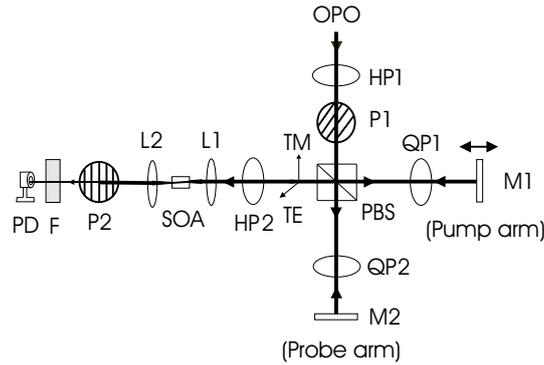
Figure 1: Schematic of the setup for nonlinear polarization switching. OPO : optical parametric oscillator, HP1-2 :half-wave plates, P1-2 : Polarizers, PBS : polarizing beam splitter, QP1-2 : quarter-wave plates, M1-2: Mirrors, L1-2 : Microscope objective lenses, SOA : semiconductor optical amplifier, F: attenuation filter, PD : photodiode
