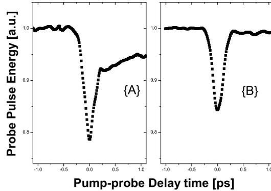
Figure 2: Pump-induced nonlinear polarization rotation. {A} corresponds to a pulse energy of 2.9 pJ while {B} to 1.7 pJ in the SOA
