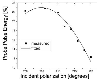
Figure 3: Pump-induced polarization rotation versus an input polarization relative to the SOA
