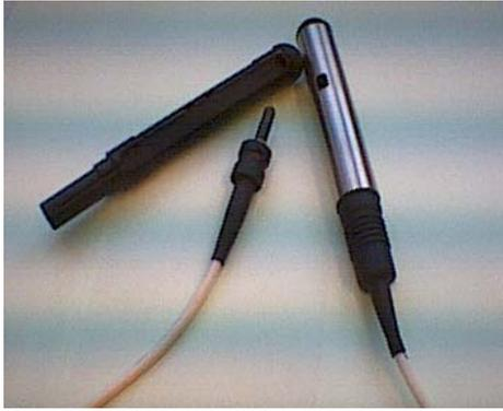
Figure 4: Photograph of the fully assembled and packaged sensor device
