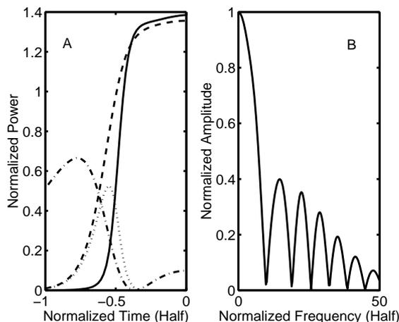
Figure 2: (a) Temporal profile of the output pulse from of a second-order cascaded NLDC, where the dashed line and solid line correspond to the 1st coupler and 2nd coupler respectively. (b) Output pulse spectrum from the launching channel of the second coupler in the second-order cascaded NLDC.
