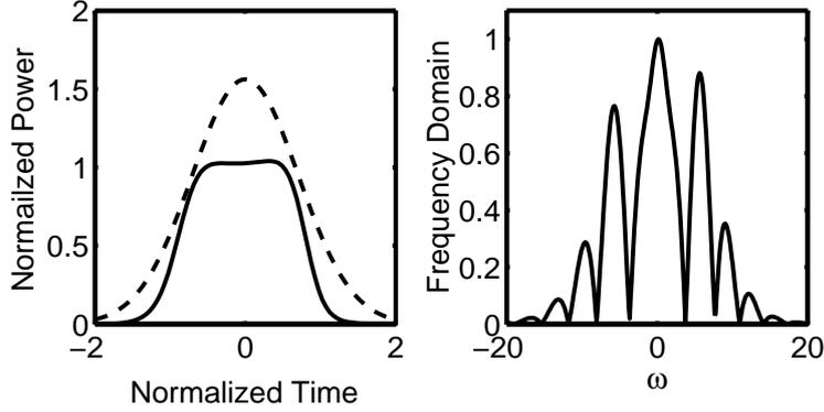
Figure 1: Pulse shape from the launching channel of a single NLDC in the time and the frequency domain.
