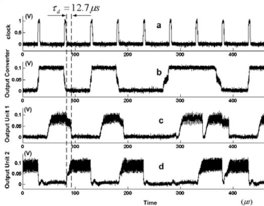
**Figure 4** experimental results of shifting the format of 01010011. a: the 20 KHz clock signal. b, c and d shows the output of the converter, Unit 1 and Unit 2 that were filtered by the filter with the center wavelength of  $\lambda_2$  (1552.92 nm), respectively.
