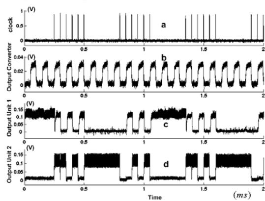
**Figure 5** experimental results when the clock format is 1111110000. a: the 20 KHz clock signal. b, c and d shows the output of the converter, Unit 1 and Unit 2 that were filtered by the filter with the center wavelength of  $\lambda_2$  (1552.92 nm), respectively.
