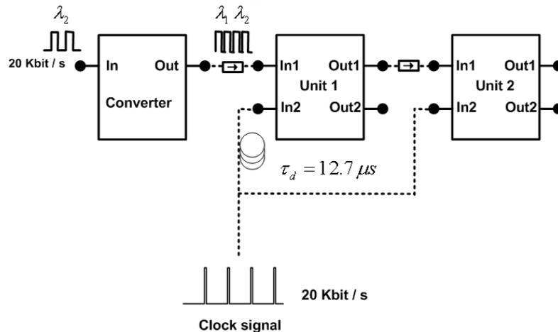
**Figure 3** the schematic configuration of optical shift register
