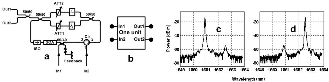
**Figure 1** a: The flip-flop memory configuration. b: The icon of the flip-flop memory. c and d show the experimental results of two stable states. ISO: isolator, ATT: Attenuator
