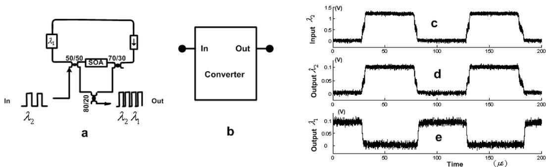
**Figure 2** a: The converter configuration. b: The icon of the converter. c: the signal injected into converter at wavelength of  $\lambda_2$  (1552.52 nm). d and e are the signal out of the converter at wavelength of  $\lambda_2$  and  $\lambda_1$  (1550.92 nm), respectively.
