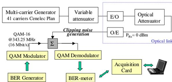
Fig. 1 – Measurement setup.
