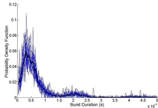
Fig. 4 – Superimposition (21 curves) of bursts duration PDF of each record. The black heavy curve corresponds to the mean of the 21 PDF.
