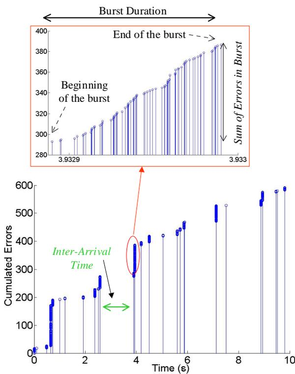
Fig. 3 – Temporal evolution of erroneous bits for the first 10 seconds of record  $\alpha$ . The inset shows a zoom of a burst.
