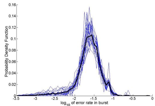
Fig. 5 – Superimposition (21 curves) of bursts error rate PDF of each record. The black heavy curve corresponds to the mean of the 21 PDF
