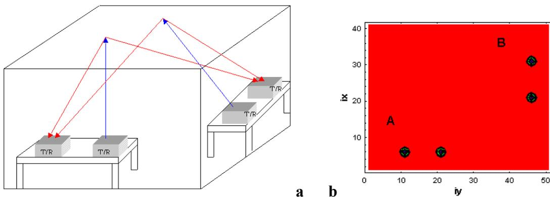
**Fig. 1:** (a) gives the sketch of a room for the IR channel model. The transmitters (T) and receivers (R) interact via the ceiling only. Figure (b) on the right indicates the positions of two specific sets (A and B) transmitter/receiver pairs on the floor of a 4x5 meter room (axes are in dm). Set A T/Rs are 1 and 3 (left to right) and Set B are 2 and 4 (top to bottom).
