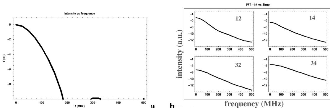
**Fig. 3.** Plots in (a) and (b) above indicate the spectrum of the total and individual channel matrices respectively. These plots are given in (intensity vs frequency- MHz). Note that the individual channel matrices have larger 3dB bandwidths that the total channel matrix.
