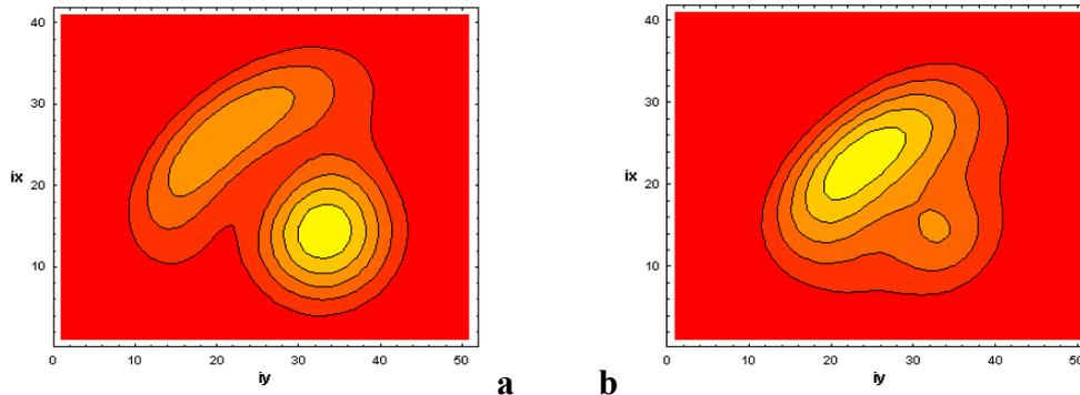
**Fig. 4.** (a) and (b) show the detected IR light pattern by set B when set A transmits a PDW beam with 150 MHz, for in- and quadrature- phase components (other parameters as in Fig.2).
