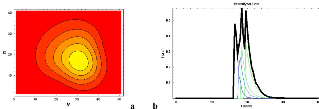
**Fig. 2.** (a) indicates the detected IR light pattern by set B when set A transmits. (b) is the impulse response for this case in (intensity vs time-nsec)
