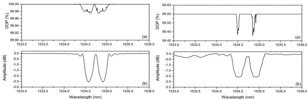
Figure 3: (a) DOP in transmission versus wavelength and (b) transmitted spectrum. Left : Simulation with  $n_{eff} = 1.4521$ ,  $\Lambda = 528.41$  nm,  $L = 6$  mm,  $\delta n = 2 \cdot 10^{-4}$  and  $\Delta n = 3.7 \cdot 10^{-4}$ ; Right : Experimental measurement
