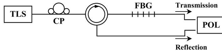
Figure 1: Measurement set-up for the DOP
