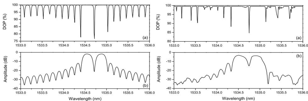
Figure 2: (a) DOP in reflection versus wavelength and (b) reflected spectrum. Left : Simulation with  $n_{eff} = 1.4521$ ,  $\Lambda = 528.41$  nm,  $L = 6$  mm,  $\delta n = 2 \cdot 10^{-4}$  and  $\Delta n = 3.7 \cdot 10^{-4}$ ; Right : Experimental measurement
