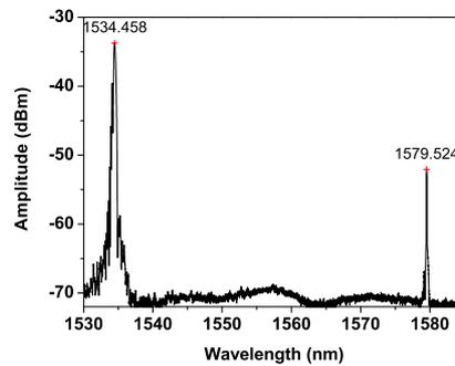
Figure 2: Reflected spectrum of the dual superimposed grating used for sensing purposes
