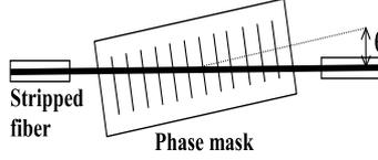
Figure 1: Rotation of the phase mask to superimpose tilted fiber Bragg gratings
