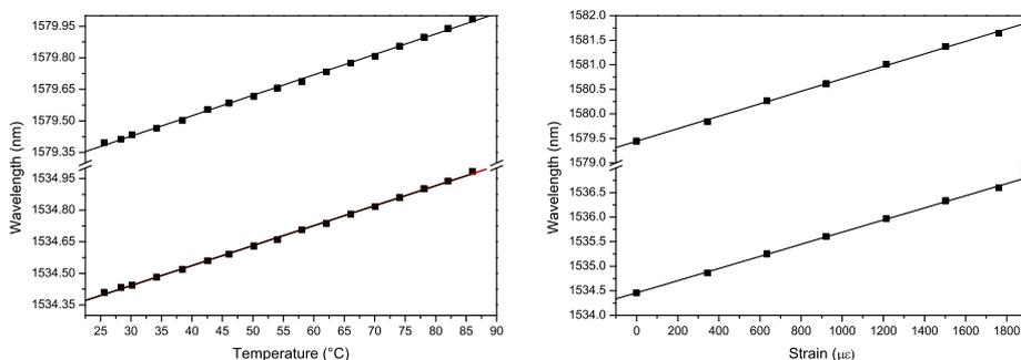
Figure 3: Wavelength shifts of the two gratings with respect to temperature and strain
