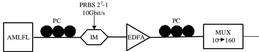
Fig.1. 160Gbit/s OTDM transmitter
