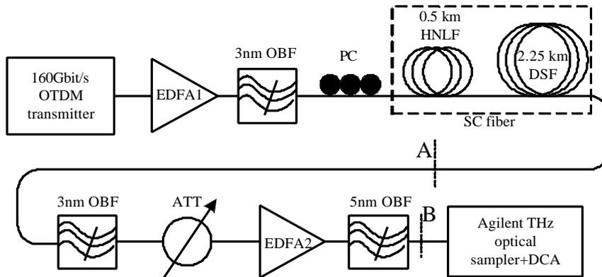
Fig. 2. Experimental setup of the multi-wavelength signal generation at 160Gbit/s
