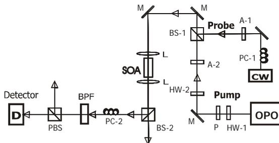
**Figure1:** Experimental setup for ultrafast wavelength conversion, where the symbols of optical components are defined as: OPO: optical parametric oscillator, HW: half-wave plate, P: polarizer, M: mirror, PBS: polarizing beam-splitter, BS: beam-splitter, L: lens, A: attenuator, BPF: band pass filter, PC: polarization controller, CW: Continuous wave tunable laser.
