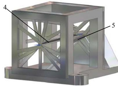
Fig. 4 Design for align fibres individually in x-y-z space by using laser support adjustment
