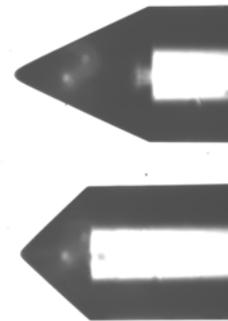
Fig.1 Lensed fibre tips with lens radii of 5 μm and tapered angles of 50° (top) and 90° (bottom).
