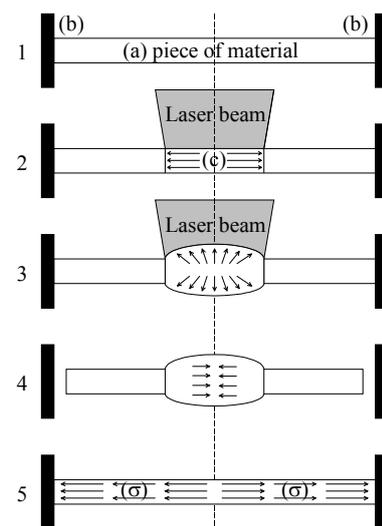
Fig. 2 Schematic presentations of laser support adjust mechanism.
