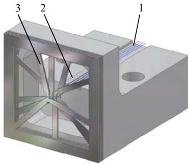
Fig. 3 Design for align fibres individually in x-y plane by using laser support adjustment
