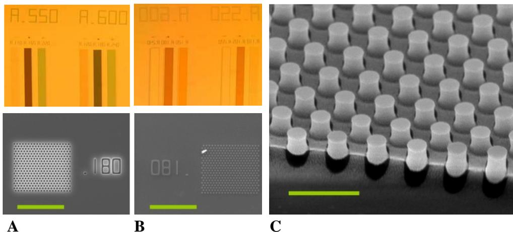
**Figure 2.** Nano imprint with a conventional Mask Aligner. The mold consists of long arrays of holes ordered in triangular lattices with different periods and pitches. A. 1 mm<sup>2</sup> of mold area and detail (bar length: 10 micron). B. 1 mm<sup>2</sup> imprint area and detail (bar length: 10 micron). C. Detail of imprint cross section (bar length: 1 micron).
