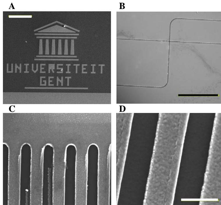
**Figure 4.** Gold patterning on silicon by lift-off after nano imprint. Dark area is silicon. A. Ghent University logo (bar length: 100 micron). B. Crossing of two 340 nm lines (bar length: 20 micron). C. Grating. D. Detail of this grating (50° tilt, bar length: 200 nm)
