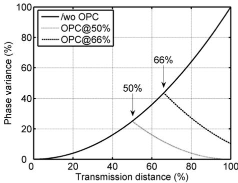
Fig. 3: Normalized phase variance due to MI-NPN as a function of the transmission distance.
