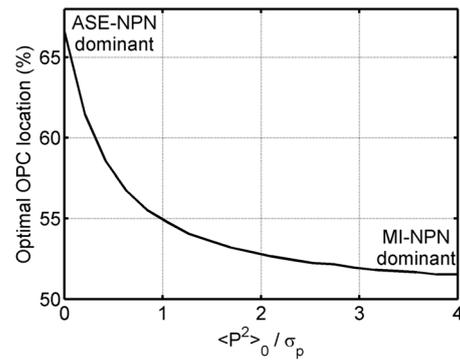
Fig. 4: Optimal OPC location as a function of the MI to ASE ratio ( $\langle p^2 \rangle_0 / \sigma_p$ )
