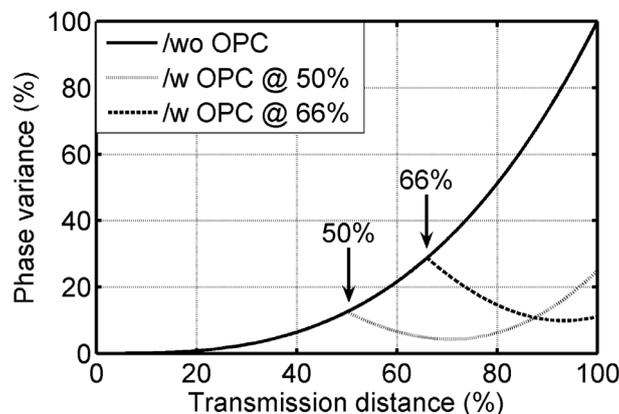
Fig. 1: Normalized phase variance due to ASE-NPN as a function of the transmission distance with (/w) and without (/wo) OPC.
