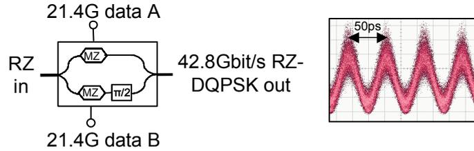
Fig. 2: Super Mach-Zehnder structure with the eye diagram of a 42.8Gbit/s RZ-DQPSK signal
