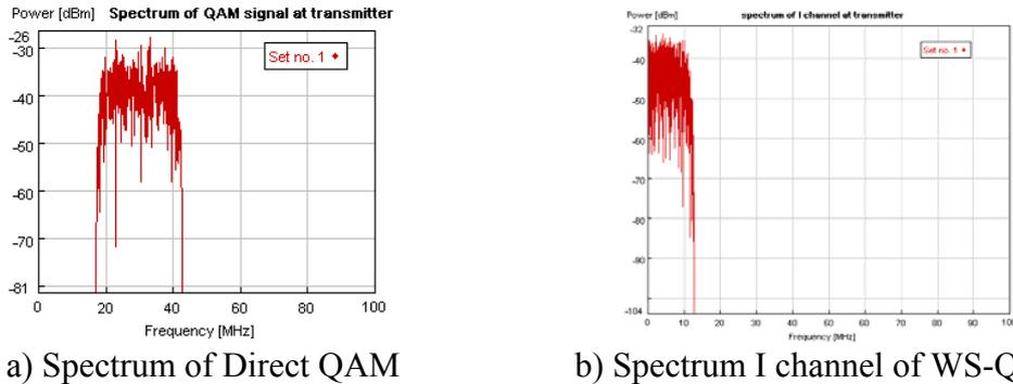
**Fig. 5 The spectrum of QAM signal after transmitter**
