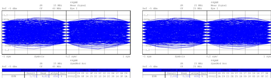
a) With 658nm laser diode, 100m POF
