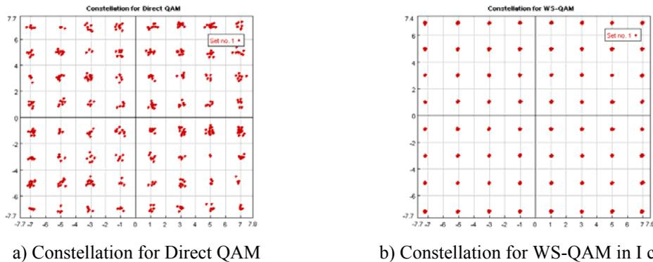
**Fig. 6 The Constellation for QAM signal after transmitter**
