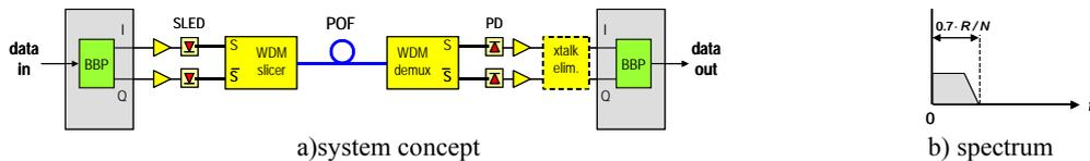
Fig. 4 Wavelength-sliced emulated QAM
