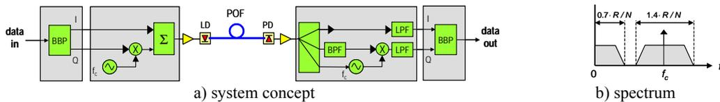
Fig. 3 Baseband/subcarrier emulated QAM
