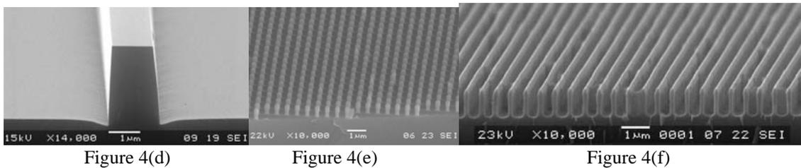
Figure 4 (d) is a waveguide of 2.3  $\mu\text{m}$  height etched in thermal silicon oxide in Alcatel Adixen DE Inductive Coupled Plasma (ICP) etching machine, using 1.2  $\mu\text{m}$  resist. It would be possible with the same amount of resist to etch around 6  $\mu\text{m}$  thermal oxide.
