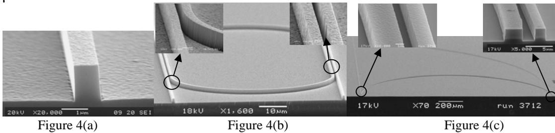
Figure 4 (c) is a micro ring resonator of 2.5  $\mu\text{m}$  height in SiON etched in the Plasmatherm 790, using resist of 0.9  $\mu\text{m}$ . The gap is around 1.0  $\mu\text{m}$ .
